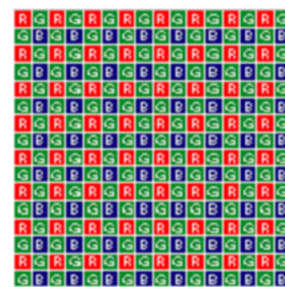
Fig. 1 Typical filter layout on CCD device
