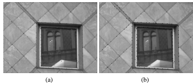
Figure 3. (a) Interest points detected with the Förstner and the Harris operator; (b) Final result after image preprocessing, application of interest operators and point filtering.
