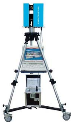
Fig. 1: 3D laser scanning system IMAGER 5003 with accessories
