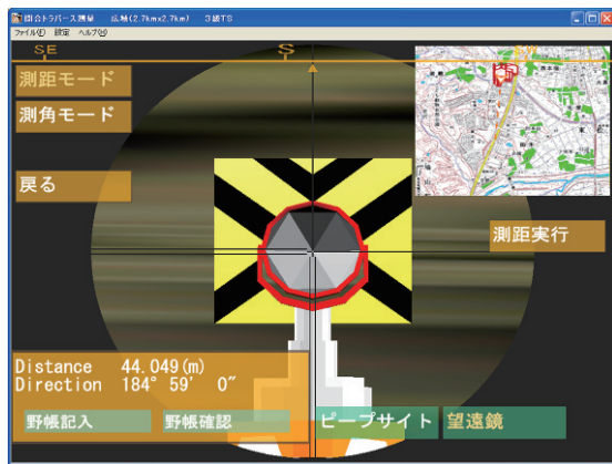
Figure 8. Collimation by telescope
