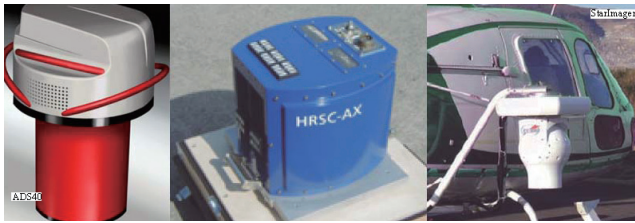
Figure.4: Airborne Linear Cameras: ADS40-HRSC-AX-StarImager
