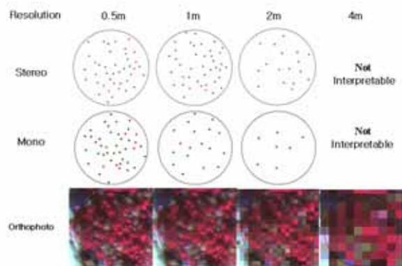
Figure 10. Trees identification in stereo and orthophoto with varying spatial resolution (Plot 2)
