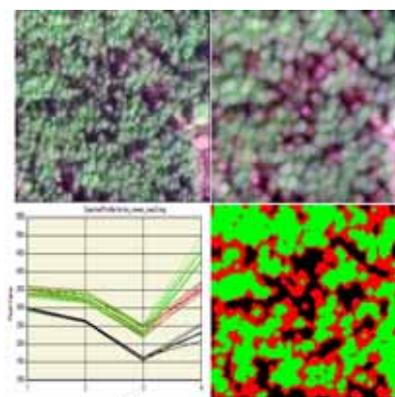
Figure 3. Original image (upper left), local\_maximum (upper right), the spectral profile (lower left), separation of damaged trees (lower right).
