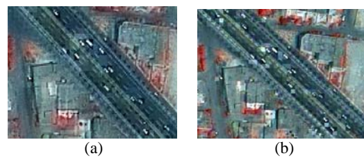
Figure 4. The wavelet-based fused data: (a) low-pass filtered fused data, (b) fused data without filtering
