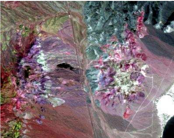
Fig. 2 Pseudo-colorful Composition (2.1 \mu m, 2.2 \mu m, 2.3 \mu m) Used To Handle AVIRIS Data of Cuprite Region (© AVIRIS Image Copyright 1995, ENVI)
