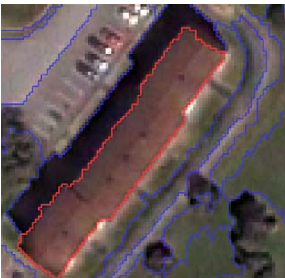
Figure 9. Extraction of high contrast building in four iterations (proposed method)
