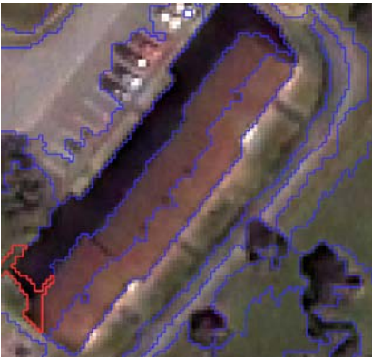
Figure 6. Sub-object of building merges with outside regions (trial and error)
