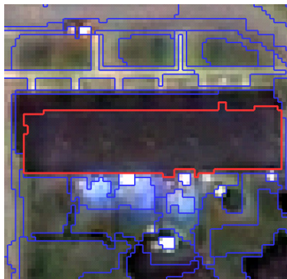
Figure 10. Extraction of low contrast building in four iterations (proposed method)
