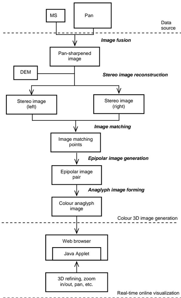
Figure 1. Flowchart of the generation of medium resolution colour 3D images from monoscopic Landsat images and the corresponding 3D online visualization
