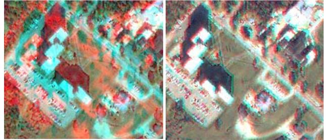
Figure 9. Influence of overall horizontal parallaxes for effective colour 3D viewing. Left: larger overall horizontal parallaxes may cause stereo fusion problems; Right: small overall horizontal parallaxes are more comfortable for colour 3D viewing.
