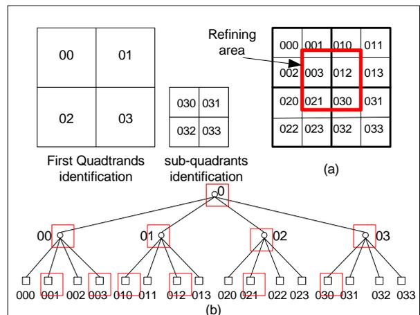
Figure 10. Quadtree method for parallax refining. (a) decomposition of an image, and (b) quadtree representation of the image.
