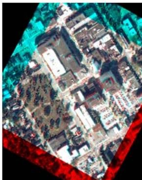
Figure 8. Colour 3D image generated using epipolar images
