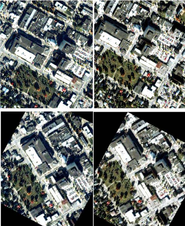
Figure 7. Epipolar geometry resampling. Top: Ikonos image pair before epipolar resampling; Bottom: epipolar images.
