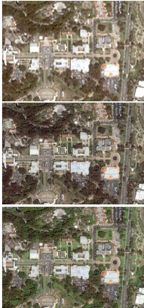
Figure 5. Colour enhancement of Ikonos natural colour image. Top: original Ikonos colour image; Middle: pan-sharpened Ikonos colour image; Bottom: pan-sharpened and colour enhanced Ikonos image.
