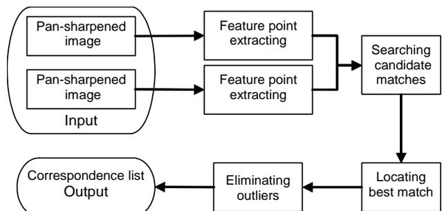
Figure 6. Overview of the image matching process involved in the colour 3D system
