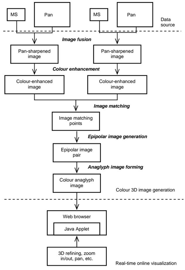
Figure 2. Flowchart of the generation of high resolution colour 3D images from QuickBird or Ikonos image pairs and the corresponding 3D online visualization
