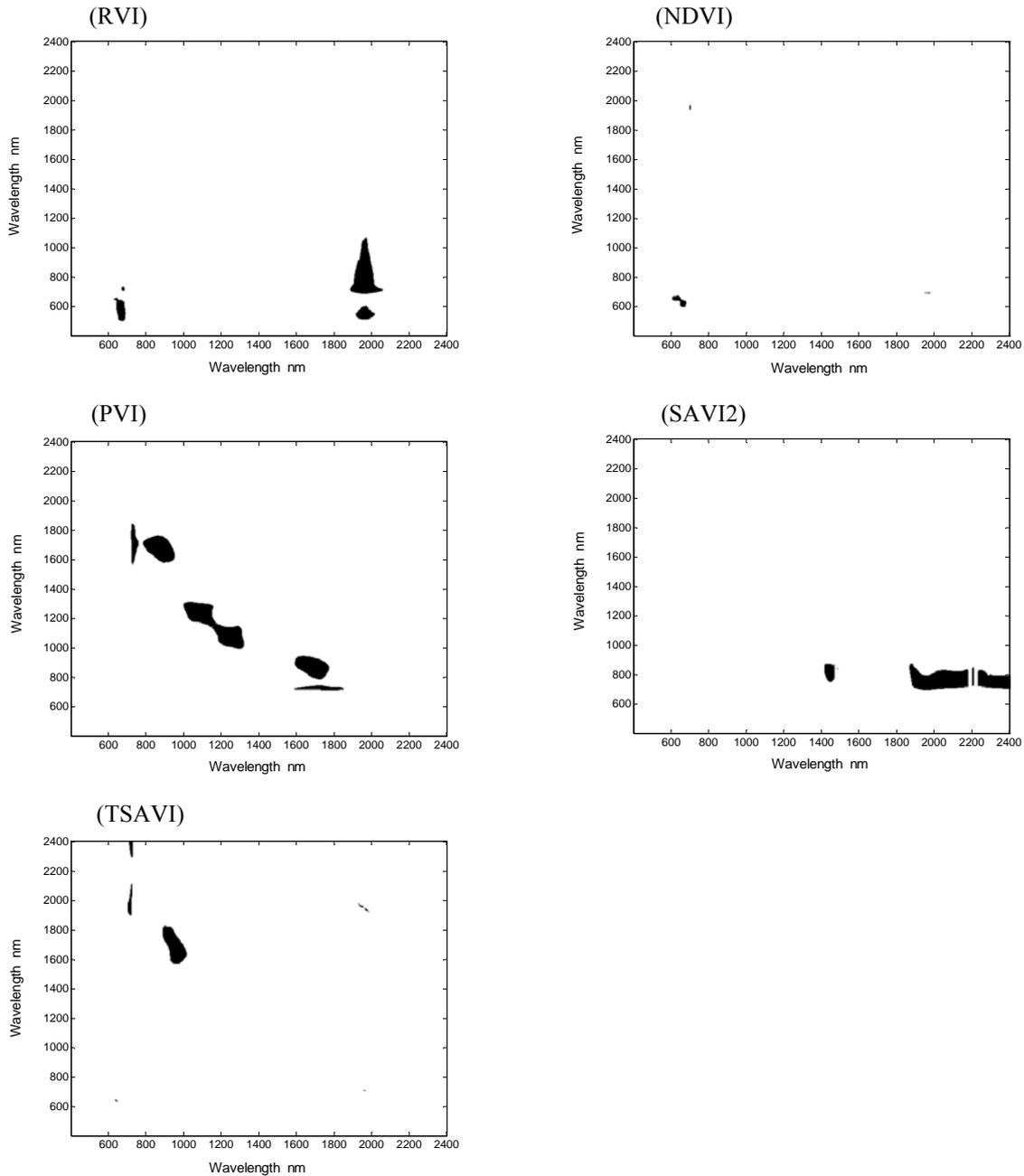
Figure 3. The “hot spot” regions where there are relatively high values of coefficient of determination  $R^2$  ( $R^2 > 0.7$ ) between band combinations and LAI. Note that only in case of TSAVI the  $R^2$  value is greater than 0.6 ( $R^2 > 0.6$ ).
