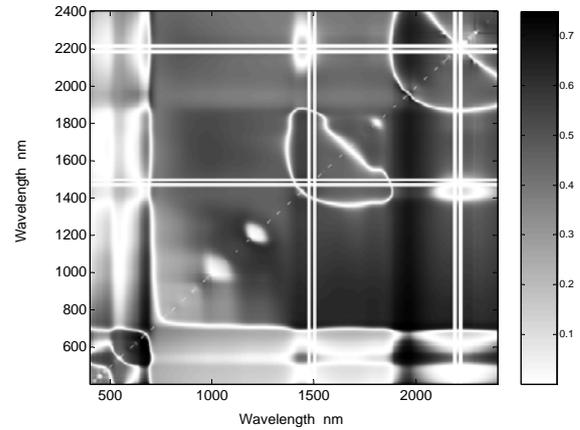
Figure 2. 2D correlation plot that illustrates the correlation of determination ( $R^2$ ) between narrow band RVI values and LAI.
