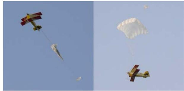
Figure 5. The landing parachute is deployed in the sky
