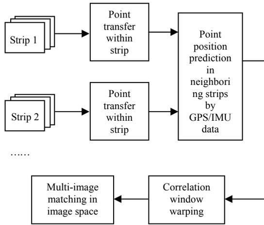
Fig.1 Workflow of point transfer method
