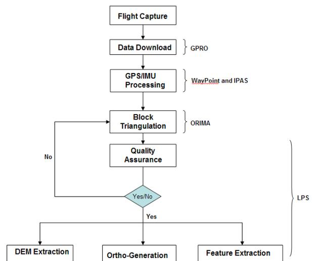
Figure 1. ADS40 Processing Workflow
