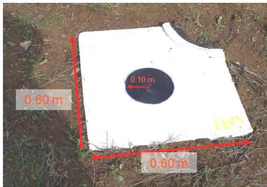
Figure 5. Presignalized target used.
