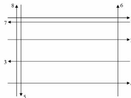
Figure 8. Configuration of strips flown at two flying heights. Strips 1 and 7, and strips 5 and 8 are double, strips with the same trajectory but with opposite directions.
