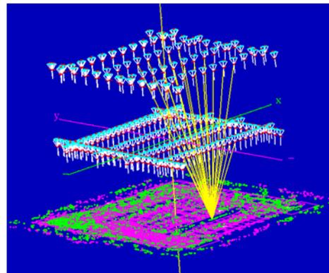
Figure 7. Calibration flight schematic representation obtained with BINGO 5.4.
