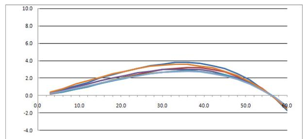
Fig. 11: Radial symmetric distortion derived from various UltraCamX test flights.
