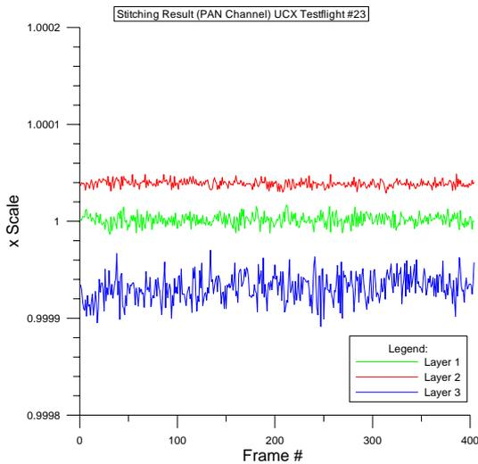
Fig 6: Stitching scales for the PAN channel (x component)
