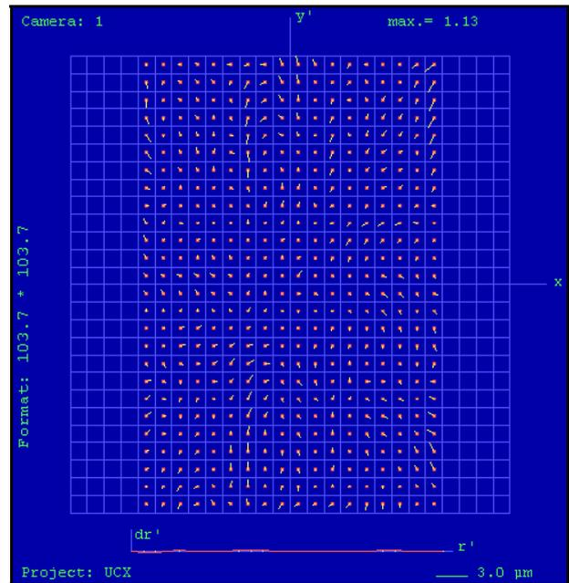
Fig. 10: Image residuals using radial distortion parameters
