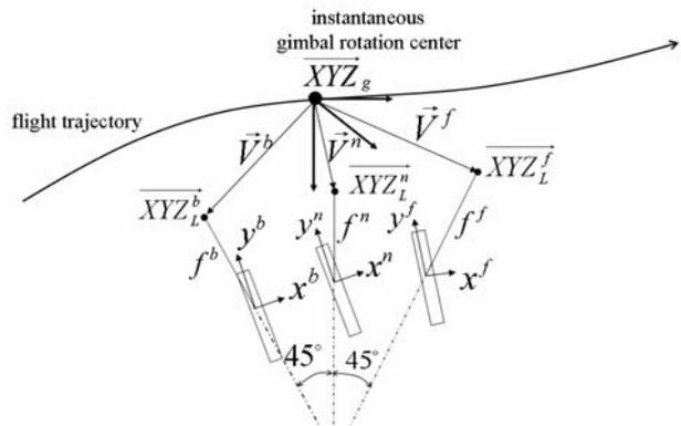
Figure 2 Imaging geometry of a three line scanner
