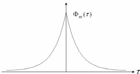
Figure 3 Autocorrelation function of 1st-order Gauss-Markov process
