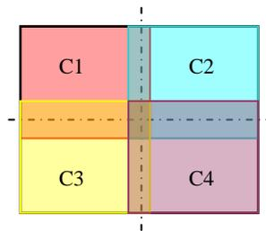
Figure 5. Four distributed CCD sensors imaging format
