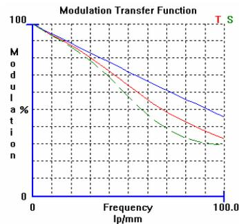
Figure 7. MTF measurement of the intercepting optical plate
