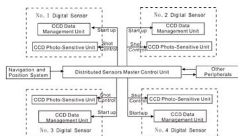
Figure 3. Four distributed CCD imaging sensors
