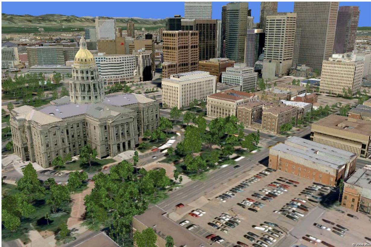
Fig. 9: Snapshot from the Virtual Earth Web Page (maps.live.com). Downtown Denver is represented by three dimensional building model with photo realistic texture. Trees are recognized by image classification and replaced by three dimensional tree models.
