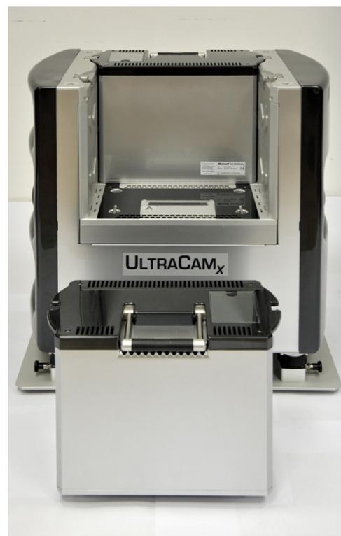
Fig. 4: UltraCamX on board computing unit and removeable Data Unit. The download of image data to the post processing station is supported by four parallel data streams of the Docking Station.
