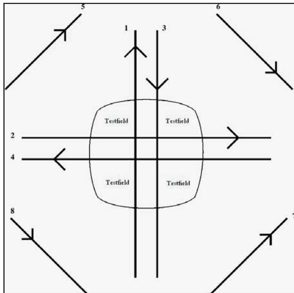
Figure 1. Schematic representation of the flight axes above the test field. Arrows represent the flight direction. Axes 1 and 3 fall together, but have been represented seperately to stress the fact that they are flown from opposite directions. The same is true for axes 2 and 4.
