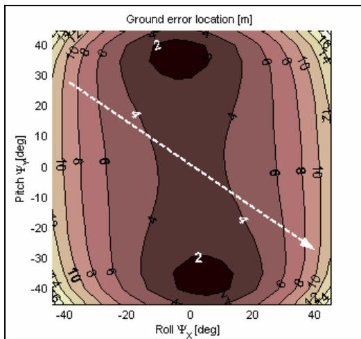
Figure 7. Ground error location after mean calibration
