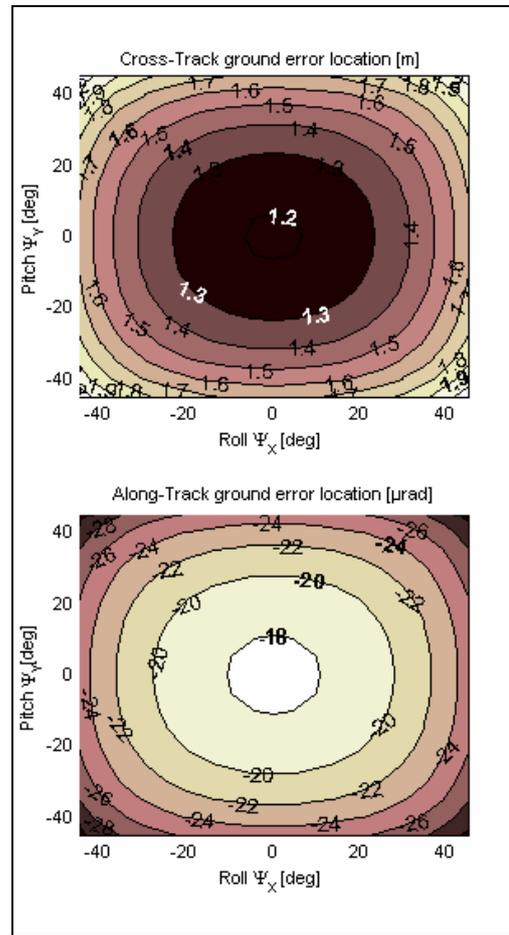
Figure 6. Ground error location components before mean calibration
