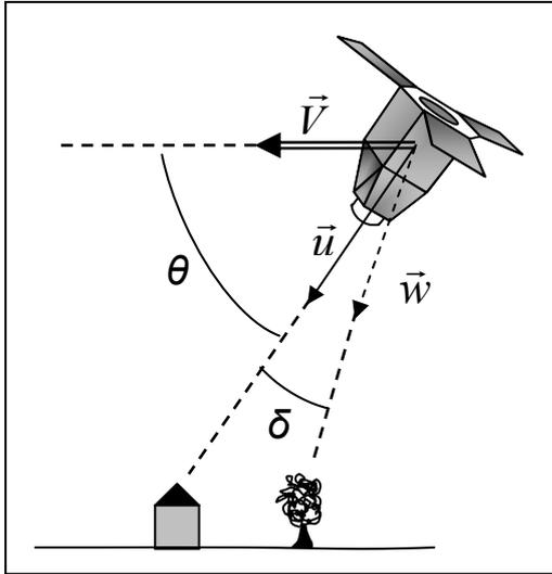
Figure 3. Aberration of light in satellite observation
