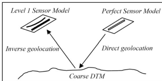
Figure 1. Perfect sensor resampling process
