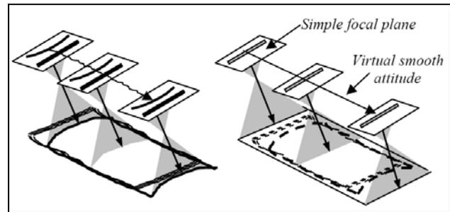
Figure 2. Perfect sensor geometry
