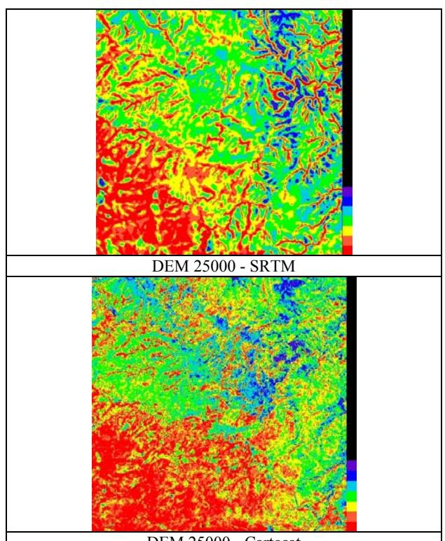
Figure 9a: colour coded differences of height models
