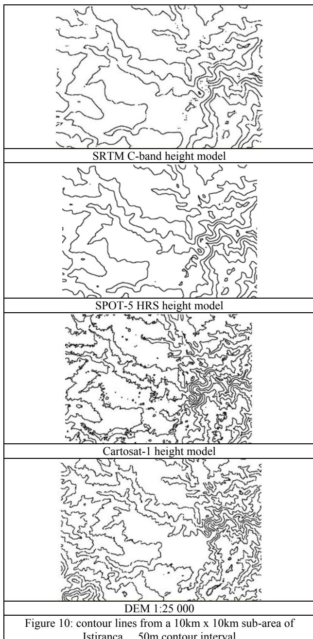
Figure 10: contour lines from a 10km x 10km sub-area of Istiranca 50m contour interval
