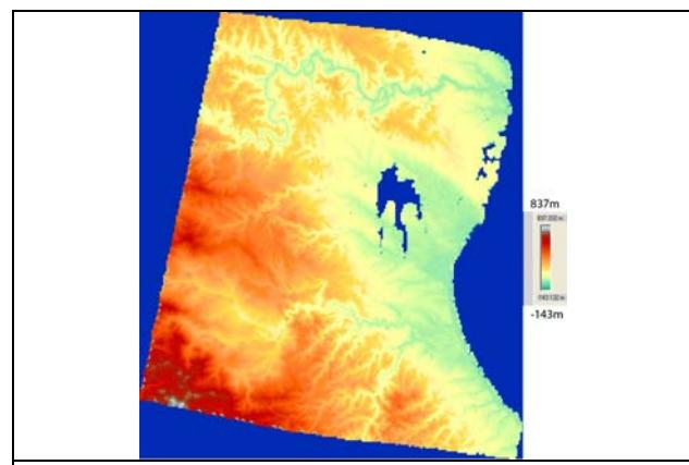
Figure 7: height model based on Cartosat-1 stereo model with height-scale
