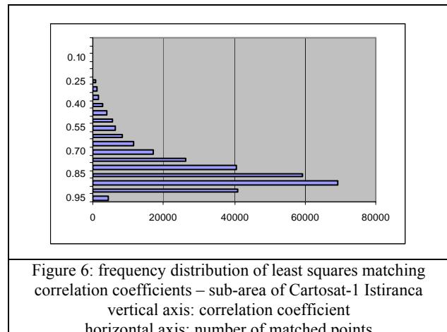
Figure 6: frequency distribution of least squares matching correlation coefficients – sub-area of Cartosat-1 Istirana
