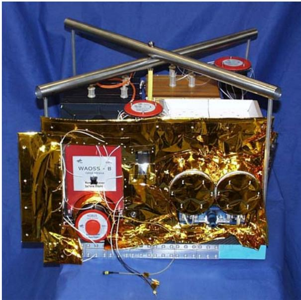
Figure 5. Micro-satellite BIRD, Mass of s/c: 94 kg, Mass of p/l: 30.2 kg
