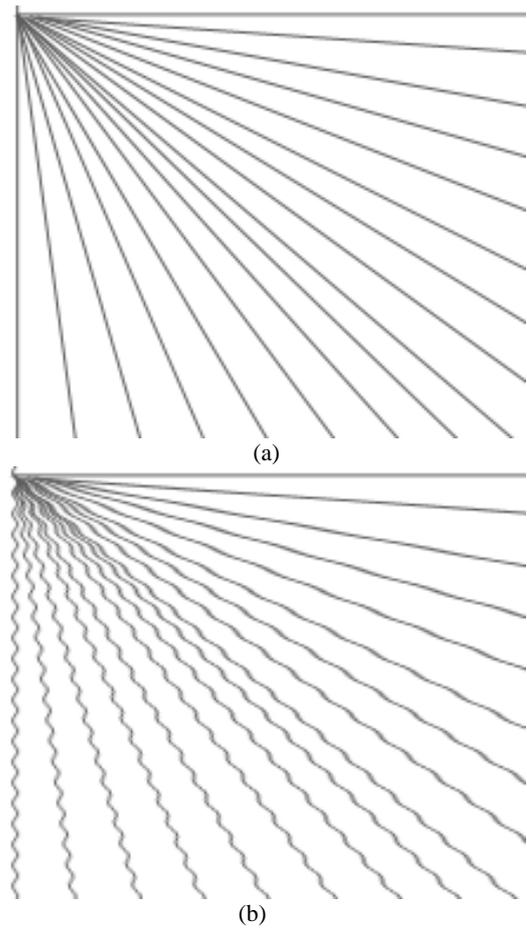
Figure 4. Jitter simulation with image containing multi-direction linear objects, where (a) is the original image, (b) is the image acquired with line jitter added
