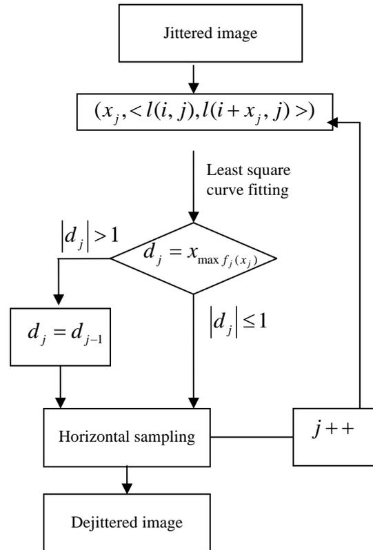
Figure 8. Process of jitter removal
