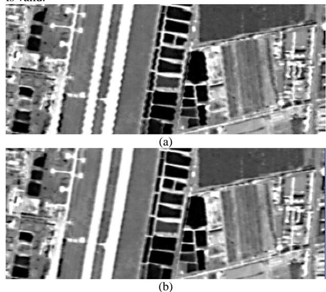
Figure 2. Jitter evaluation with image of an airdrome, where (a) represents the jittered image, (b) represents the image after shifting and sampling of whole lines
