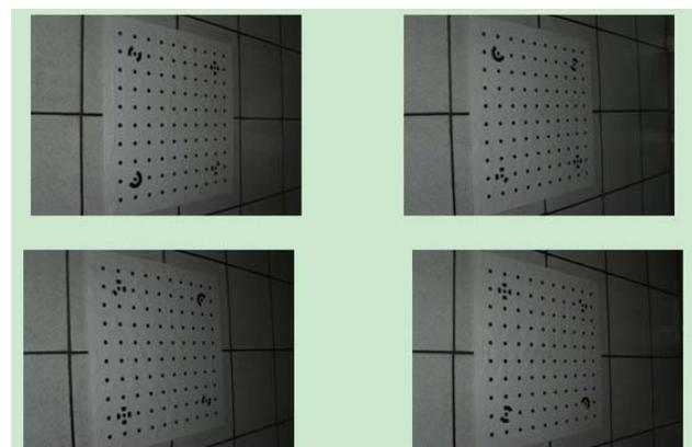
Fig.2 The second four images of the model plane. They are photographed with the camera rotated 90 degrees anti-clockwise.
