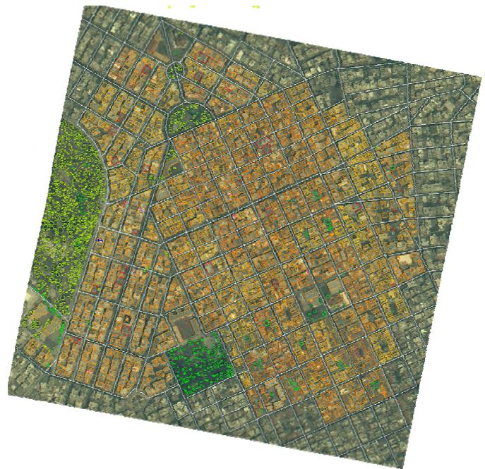
Figure 13. Orthorectified section from the Athens scene (UTM projection) with manually marked trees (green circles) and building outlines (orange polygons)
