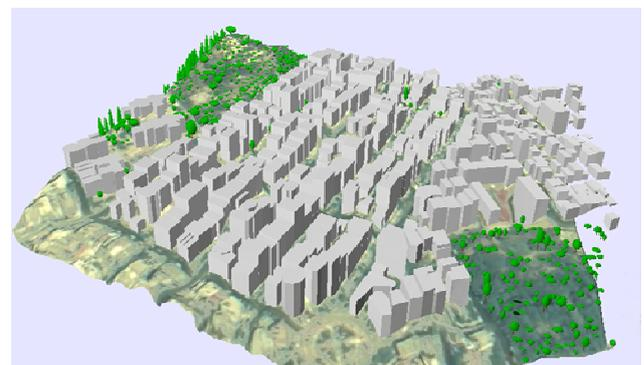
Figure 14. 3D view automatically generated from the DSM and the manually marked trees and building footprints from the Athens scene, size 500 m x 500 m
