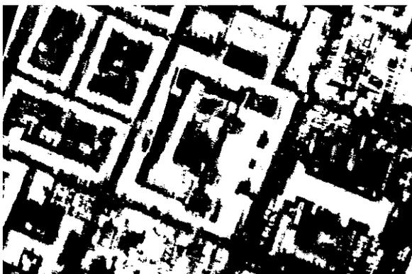
Figure 9. High objects mask calculated from the nDEM applying a height threshold of 4 m (section 600 m × 400 m)
