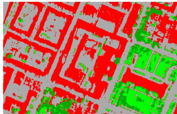
Figure 11. Classification of the Munich scene using a height mask derived from nDEM and a vegetation mask based on the NDVI from the pan-sharpened orthophotos
