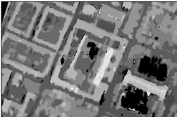
Figure 5. Digital surface model calculated for a section of 600 m × 400 m from the Munich scene using the “dynamic line warping” approach
