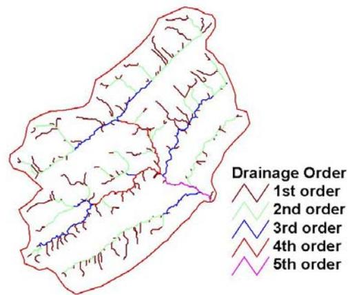
Fig. 7a Drainage Network extracted from 5m DEM
