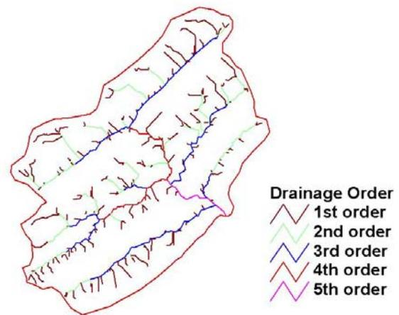
Fig. 7b Drainage Network extracted from 10m DEM
