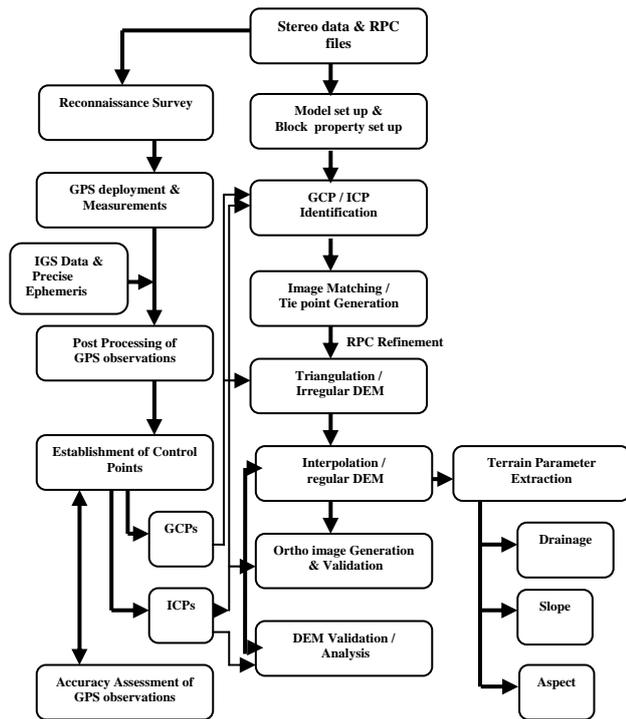
Figure 1. Methodology flowchart for stereo data analysis, validation and extraction of terrain parameters
