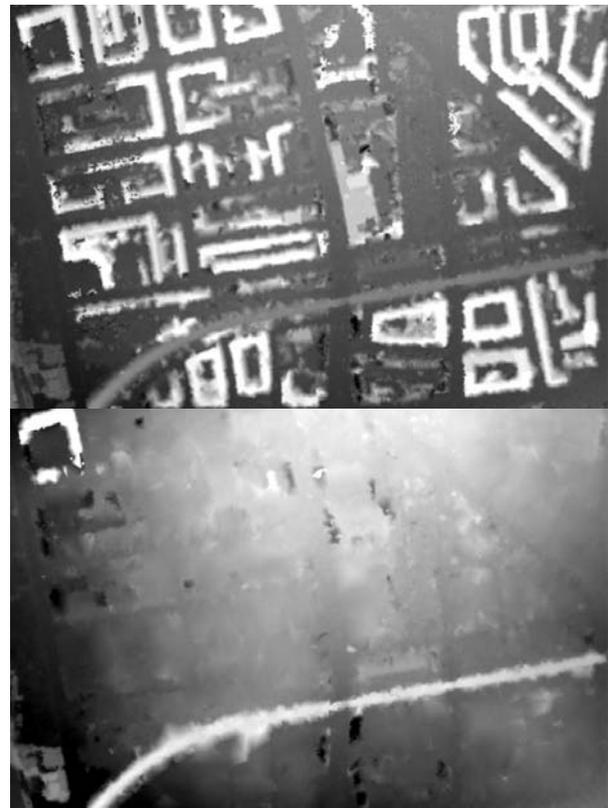
Figure 5. DSM before (above) and after (below) object filter
