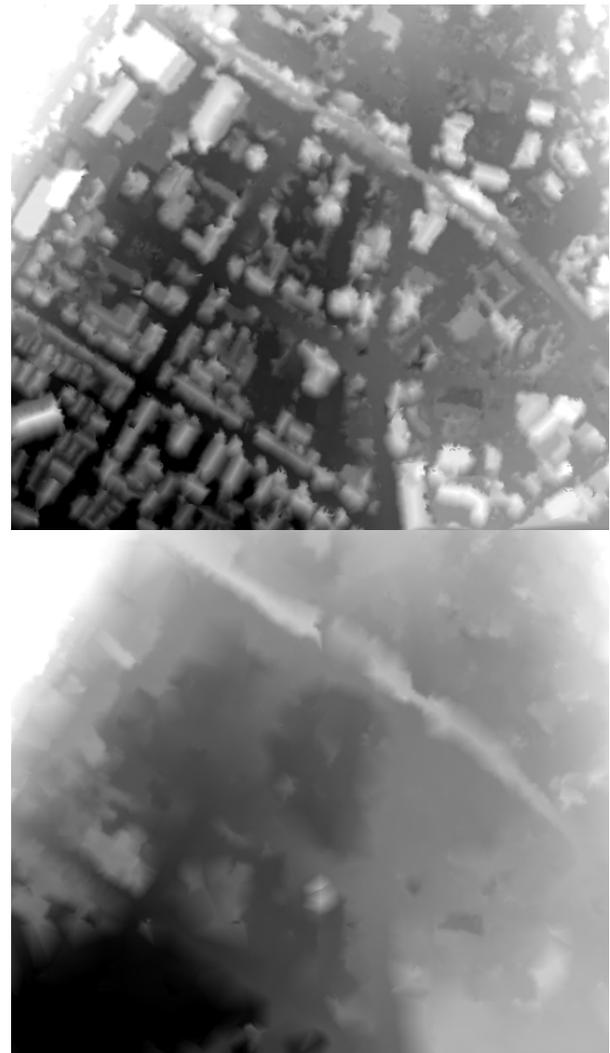
Figure 11. DSM (above) and DTM (below) from ADS40
