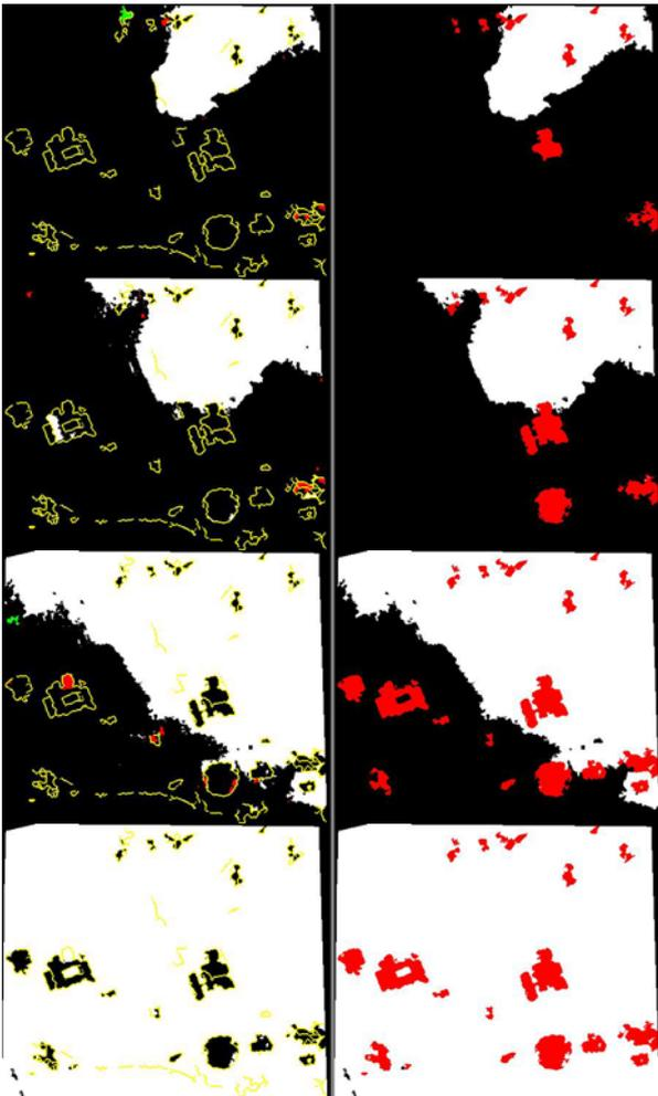
Figure 4. Status at elevation levels 277.4m, 272.4m, 265.4m, 252.2m, ordered from top to bottom. Legend: white (terrain), black (under water), yellow (slope edge), red/green (new isolated regions). Right: white (extracted terrain), red (filtered objects)
