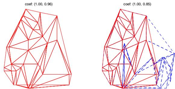
Figure 1. Positional correlation coefficients without blunders (left, vertex linked by solid lines) and with blunders (right, points linked only by dashed lines). Points are triangulated in objected space and linked in image space to show the displacement
