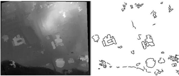
Figure 3. DSM (left) of a test region and corresponding slope edges (right)
