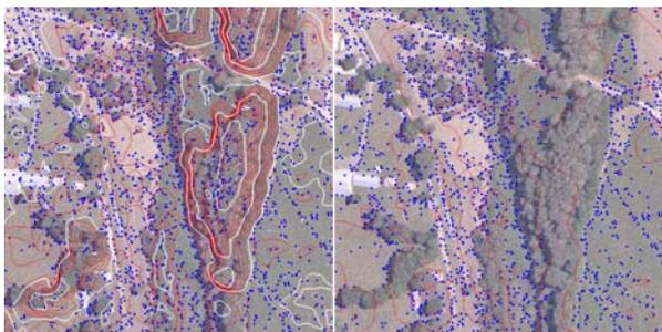
Figure 7. Points and contours before (left) and after (right) object filtering
