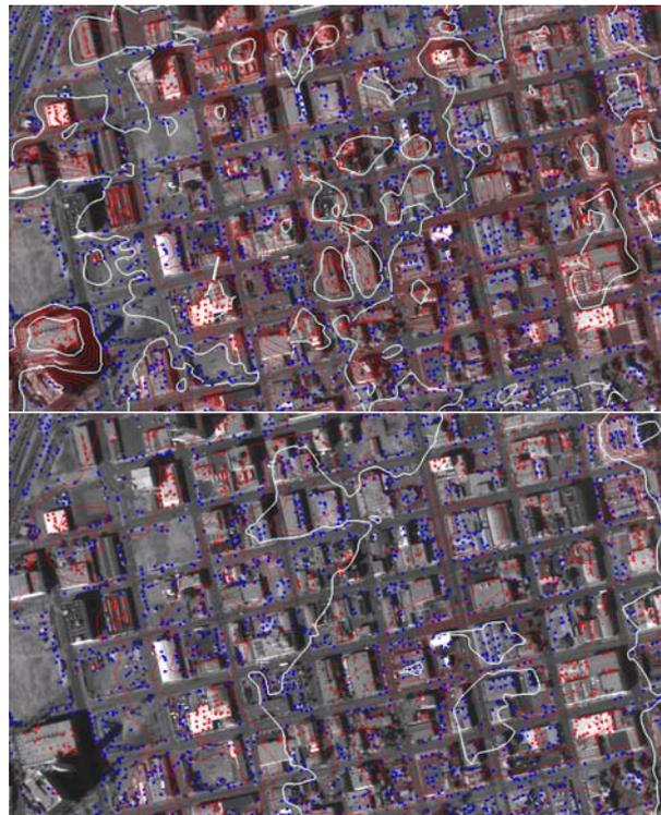
Figure 9. IKONOS image overlapped with extracted points (red: points on objects; blue: points on ground) and contours, before (above) and after (below) object filtering
