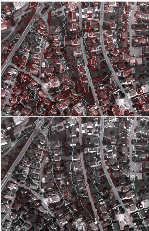
Figure 10. Contours overlapped with ADS40 images, before (above) and after (below) object filtering
