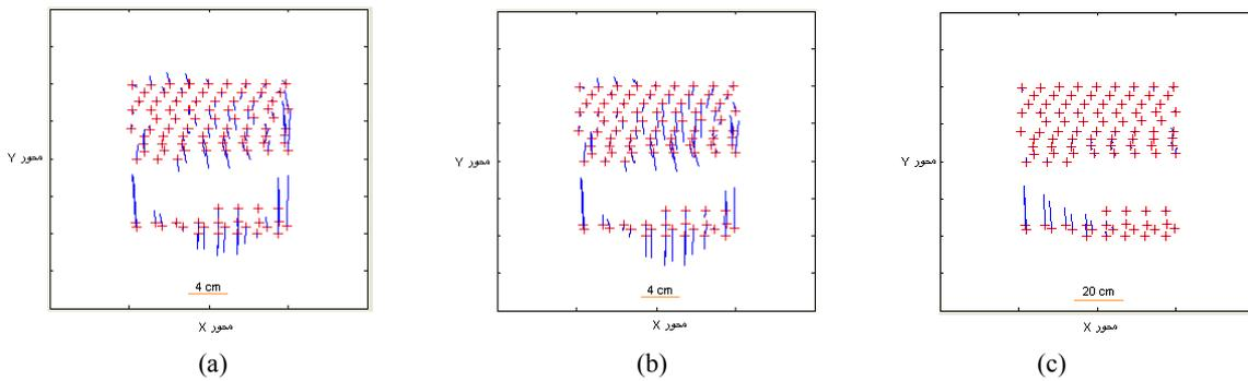
Figure 11. Planimetric error vectors of first order rational functions in a) optimum sampling b) over sampling c) under sampling
