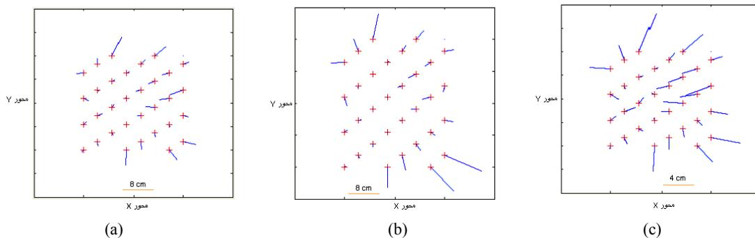
Figure 6. Planimetric error vectors of first order rational functions in a) optimum sampling b) over sampling c) under sampling
