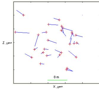
Figure 13. Planimetric error vectors of first order rational functions
