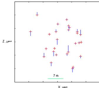
Figure 14. Height error vectors of first order rational functions
