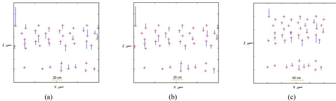
Figure 12. Height error vectors of first order rational functions in a) optimum sampling b) over sampling c) under sampling
