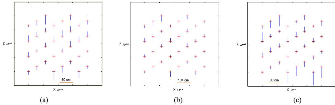
Figure 7. Height error vectors of first order rational functions in a) optimum sampling b) over sampling c) under sampling
