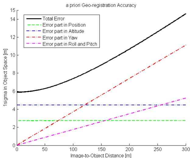
Figure 7: A priori estimate for the achievable direct geo-registration accuracy with the micro UAV 'microdrones md4-200'
