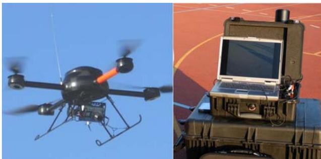
Figure 1: Quadcopter micro UAV (microdrones md4-200) system (left) with portable ground control station (right)
