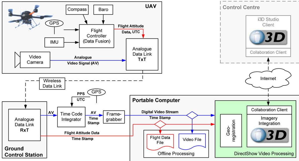
Figure 5: System architecture and data processing chain of the video imagery integration
