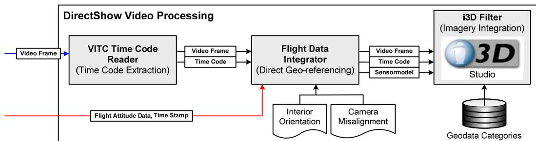
Figure 6: Filter graph for video processing
