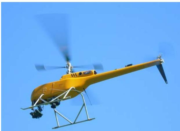
Figure 1. Geocopter's Photogrammetric UAV
