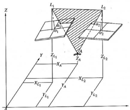
Figure 2. The coplanarity condition (Wolf et al., 2000)
