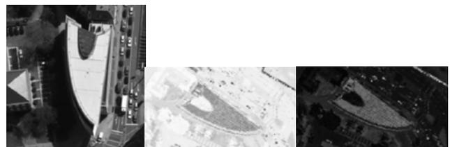
A) Aerial image, Negative LiDAR Intensity, Positive LiDAR
