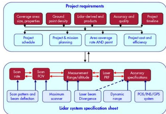
Figure 1. Matching performance characteristics from the lidar specification sheet to project requirements
