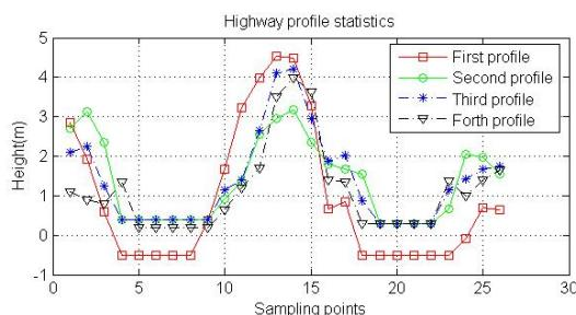
Figure 3. Highway's profile sampled on different sections
