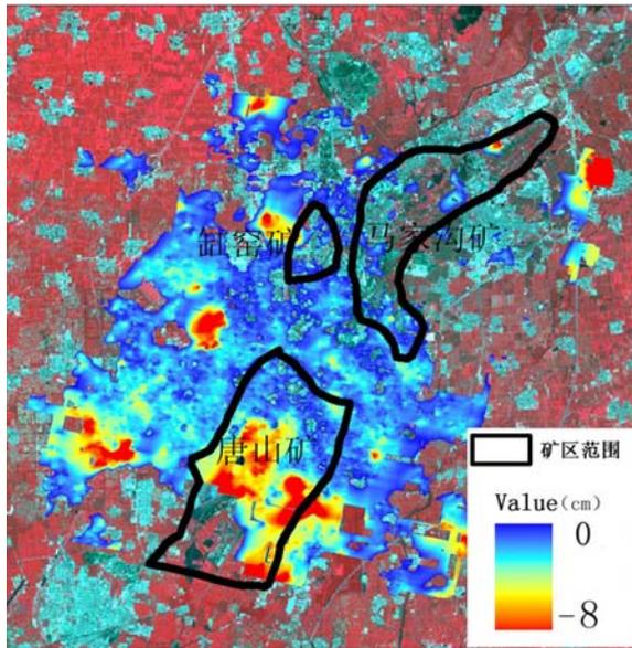
Figure 5 Subsidence 1998.5-2000.5. ETM (1999, band: 321) image is shown in the background, and overlapped with the mine area map. The largest displacement is 8cm in Tangshan mine area, in Gangyao mine and Majiagou mine, it has averagely 1 cm displacement, and in west of Tangshan mine area, and it has averagely 3 cm displacement due to the Kast collapse.
