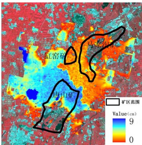
Figure 3 Subsidence 1996.1-1997.10. The subsidence regions can be seen clearly and the color coding indicates the magnitude of subsidence. TM (1999, band: 321) image is shown in the background, and overlapped with the mine area map (solid black line). The largest displacement is 9cm in West of Tangshan, In Tangshan Mine area, it has averagely 7cm displacement, in Gangyao Mine and Majiagou Mine, and it has 1.5cm displacement.
