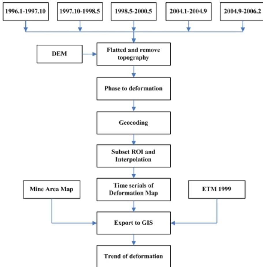
Figure2 Subsidence monitoring method based on time series of interferograms
