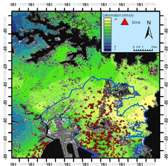
Figure 8. Deformation result using PSInSAR
