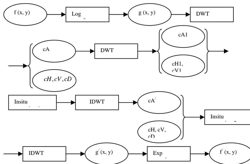
Figure1. Fundamental flow of proposed method
