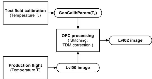
Fig. 7: Stitching process with integrated TDM correction
