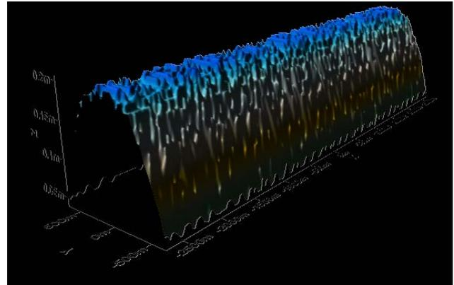
Fig. 13: Simulation of a single strip (30 images, 80% overlap). Systematic DTM errors caused by a simulated radial distortion using correct EO parameters.
