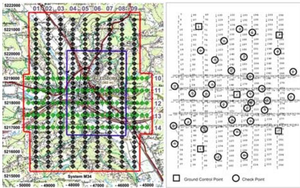
Fig. 4: Test area near Graz, Austria. Flight plan with 14 flight lines (404 images).
