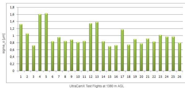
Fig. 5: Sigma\_o values obtained from the automatic aerotriangulation of several UltraCamX test flights at 10 cm GSD (1380 m AGL).
