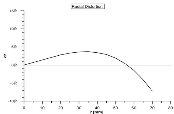
Fig. 11: Radial distortion curve (3.5µm at 35mm)
