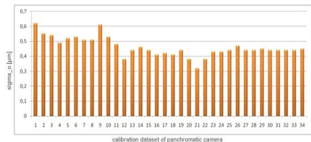
Fig. 3: Results of the bundle adjustment after the estimation of camera parameters (panchromatic camera).
