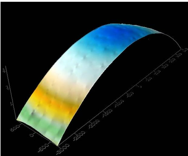
Fig. 12: Simulation of a single strip (30 images, 80% overlap). Systematic DTM errors caused by distorted EO parameters (Z-values).
