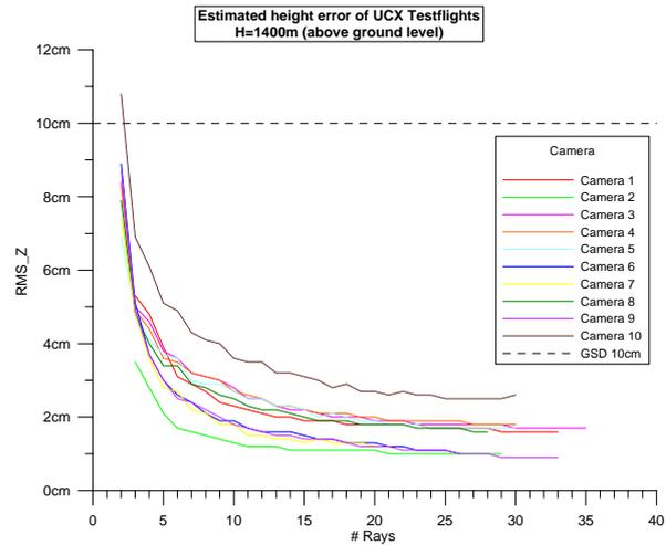
Fig. 10: Estimated height errors and number of rays
