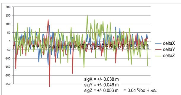
Fig. 6: Check point residuals after the bundle adjustment.
