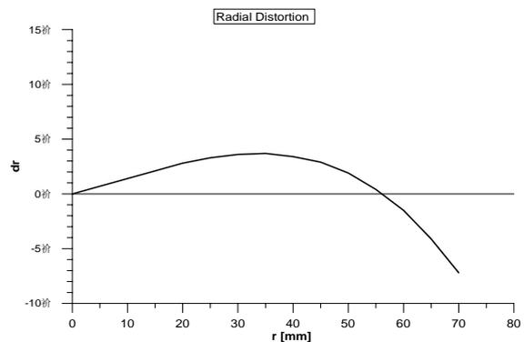
Fig. 11: Radial distortion curve (3.5µm at 35mm)
