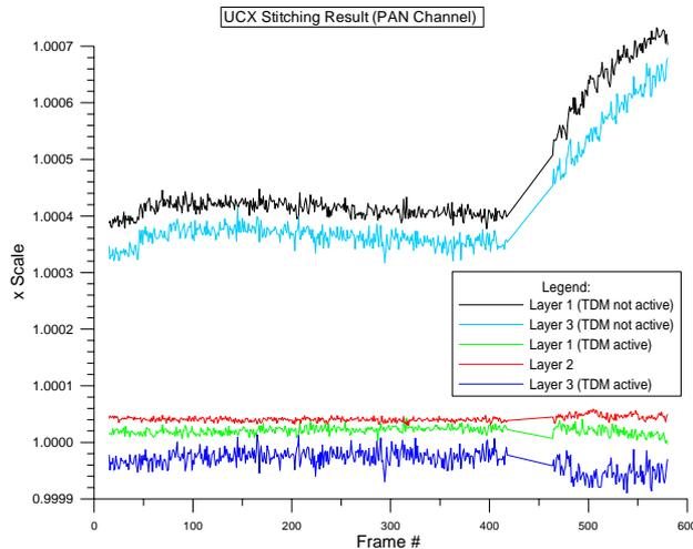
Fig. 9: Stitching scales before and after TDM correction
