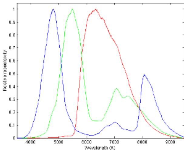
Figure 3. Spectral sensitivity of unfiltered Canon 350D sensor.
