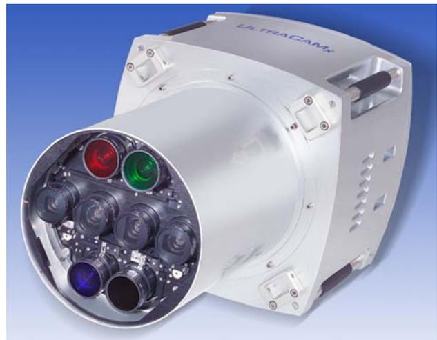
Figure 1 – Sensor head of UltraCam X digital aerial camera system with 8 cones and five spectral bands (pan, RGB and NIR). The multi spectral cones are equipped with color filters.
