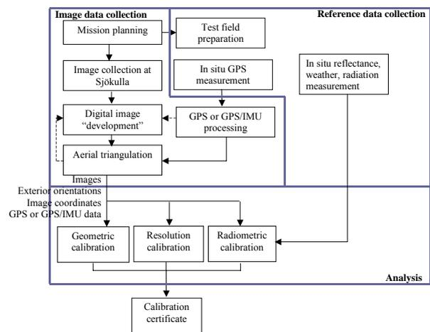
Figure 2. Test field calibration process flow (Honkavaara, 2008).
