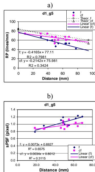
Figure 4. Analysis of a) RP and b)  $\sigma_{PSF}$  as a function of the distance from the image center. (f: flight and cf: cross-flight direction)
