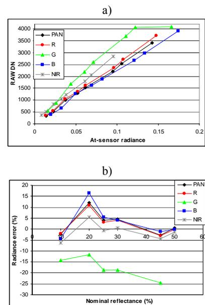
Figure 5. DMC radiometry evaluation, GSD=5 cm. a) DN's plotted as a function of at-sensor radiance. b) Absolute calibration residuals as a % of radiance, 5% and 70% targets were used as a reference (5% and 50% for green channel).
