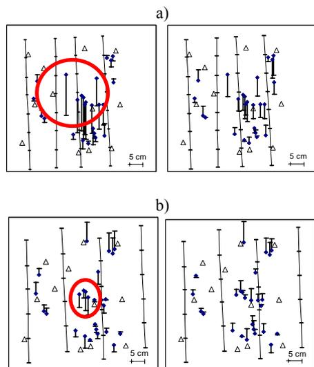
Figure 3. Errors at independent checkpoints in height coordinates: a) UltraCamD, GSD=4 cm. b) DMC, GSD=5 cm. Left: no self-calibration, right self-calibration using single-head physical parameters.
