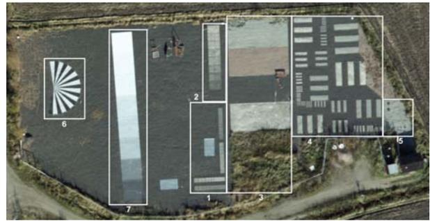
Figure 1. The Sjökuilla image quality test field: 1) permanent dense resolution bar target, 2) permanent gray scale, 3) permanent reflectance targets, 4) sparse resolution bar target, 5) permanent circular targets, 6) portable Siemens star, and 7) portable gray scale.
