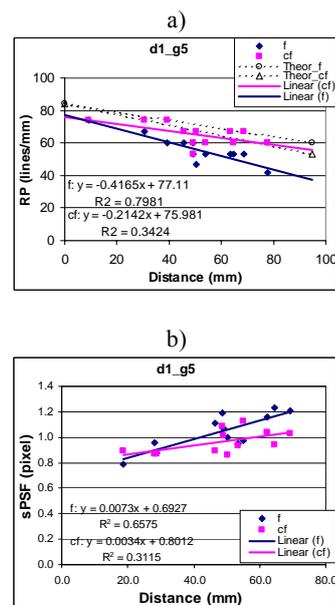
Figure 4. Analysis of a) RP and b)  $\sigma_{\text{PSF}}$  as a function of the distance from the image center. (f: flight and cf: cross-flight direction)
