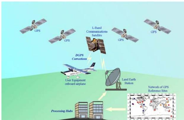
Figure 8. Satellite Based Augmentation Services
