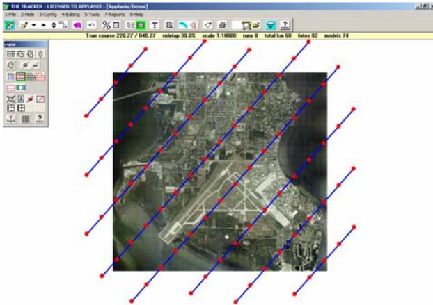
Figure 3. Flight planning example using XTRACK
