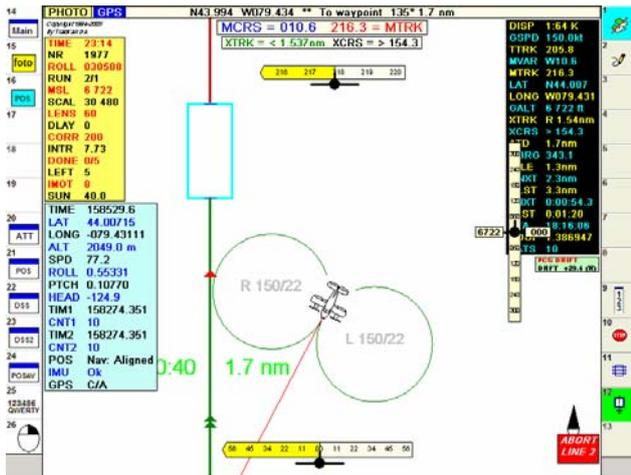
Figure 6. Turn Circle for flight guidance
