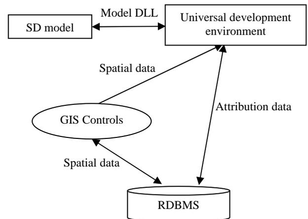
Figure 2. The integration framework of Component GIS and SD embedded software development kit
