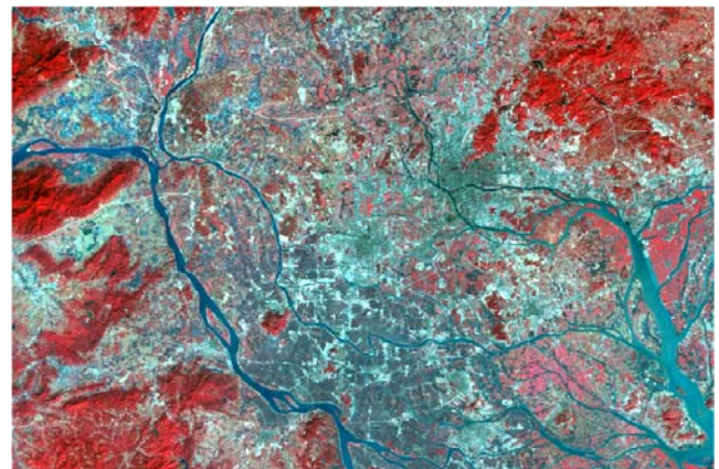
Figure 1. The experimental image of TM in color composite with bands 4,3,2 in R,G,B
