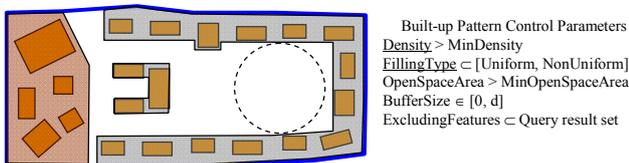
Figure 5. The Built-up pattern specification (manual drawing)
