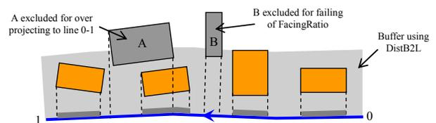
Figure 8. Aligning by projecting
