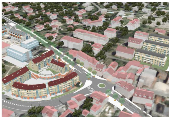
Figure 7. Different LOD of representation of buildings suggested within the case study of Collonges-Bellerive district, for the integration and visualization of new architectural projects (source: DCMO, Geneva)
