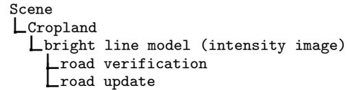
While line extraction for road update is carried out for the whole context region line extraction for road verification is done for each road object separately. More precisely, the line extraction uses the road object specific parameter road width, given in the MGCP database, within a buffer around the vector representing the road axis. The buffer width complies with the road width attribute and the nominal accuracy of the MGCP road objects being 25m.
