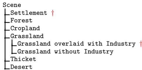
On the first level a Top-Down operator separates the IKONOS scene along appropriate context regions based on the available information of given MGCP database. The marked nodes (†) for settlement and industry are not used for the road extraction process.
