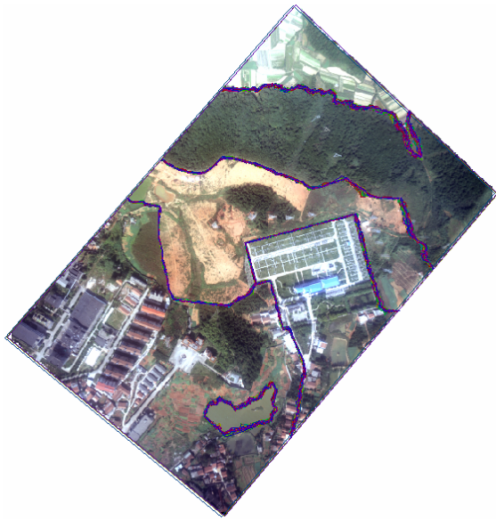
Figure 5. 100 simulated DLGs overlaid on reference DOM. Based on the error DLGs, areas and perimeters of every polygon formed with boundaries were calculated. And then the standard deviation of 100 DLGs were obtained by mathematical statistics (in Table 1)
