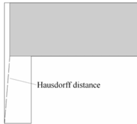
Figure 1. Hausdorff distance between the initial and generalized polygons
