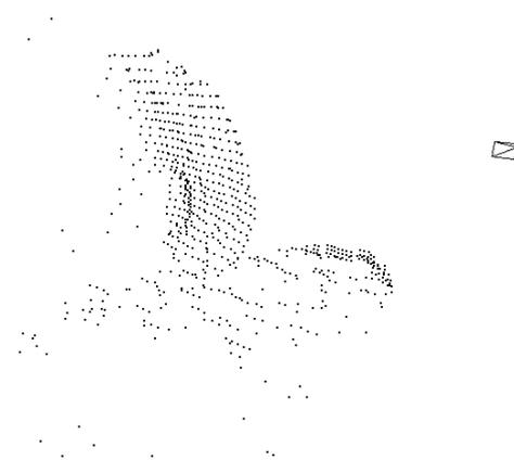
Figure 4: Camera pose and 3D point cloud obtained only from the first depth image. The image is showing a view of the office chair from behind and toward the camera. The point cloud is still very sparse comprising of only 3072 points.
